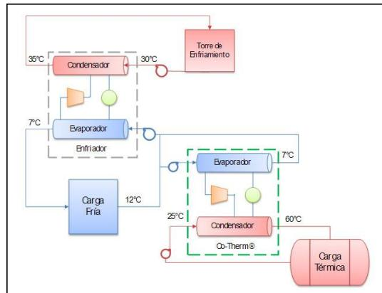
**Figure 2.** - This diagram depicts a typical interface of a Co-Therm machine with an existing chiller. The Co-Therm Fluid Heater developed and manufactured by TECSIR of Mexico is a machine using either HCFC22 or HFC134a that maintains 60°C water in the hotel water tanks. This machine replaces the duty of boilers and gas water heaters. The 2006-2008 market test in Puerto Vallarta Mexico had the machines installed in eight hotels using HFC 134a.
