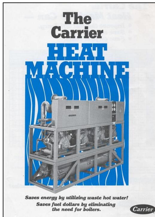
**Figure 1** - In the 1980's air conditioning manufacturers such as Carrier developed vapor compression machines using HCFC22 and CFC12 that produced hot water thereby recovering a buildings internal heat instead of burning fuel in boilers.
